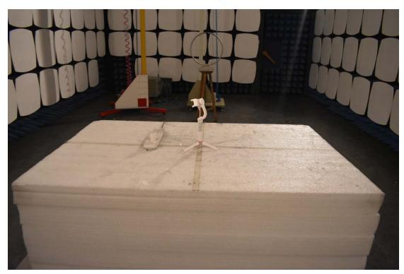
3. Radiated emission (9KHz-30MHz)
