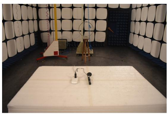
3. Radiated emission (9KHz-30MHz)
