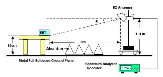
Note: The Horn Antenna maintaining bore sight alignment.
