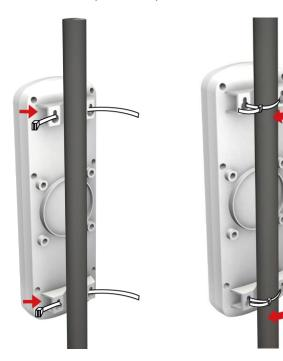
Mounting and Radio forward Diagram
