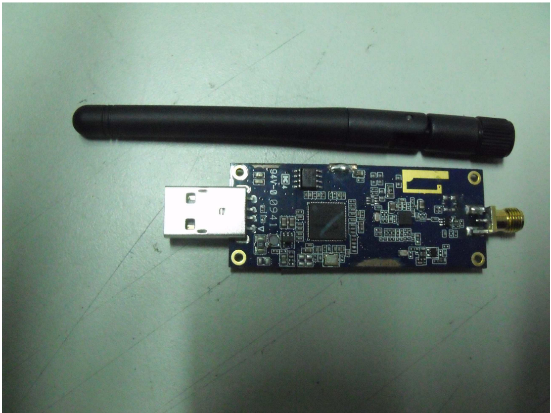
Antenna is un-detachable, reverse SMA type.
