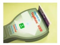
The first configuration is optimal for desktop operations, and does not obscure the LED. The second configuration, an "end-on" read mode, may be optimal for processing tags that are hard to reach, since the reader may be extended farther and more ergonomically to reach the tag. For end-on reading, positioning of the tag so that about half of it extends above the upper surface of the reader, as shown above, will give better results than completely centering the tag on the end of the reader.
