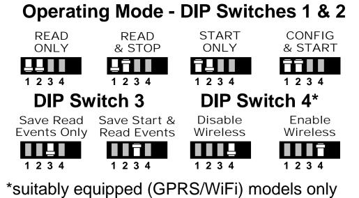
In addition to the main operating mode settings, which are controlled by the first two
