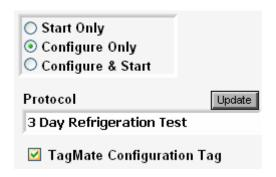
With this option selected, a tag presented to the reader will be specially marked as a TagMate<sup>®</sup> Configuration Tag, and the protocol name (first 16 characters) will automatically be placed in the Info field. The compelte set of configuration parameters that appear in the Time and Temperature panels of the software screen will be written to the TagMate<sup>®</sup> Configuration Tag and trsnferred to the TagMate USB<sup>®</sup>.
