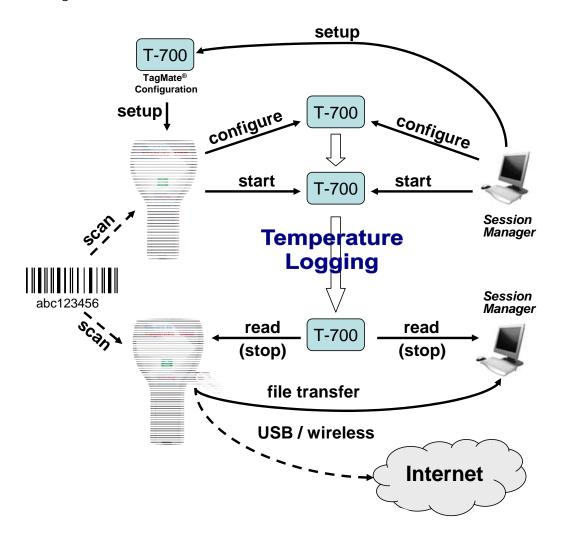
TagMate USB® can be combined with hosted solutions for pre-configuration and recycling of T-700 tags, and global data access via the Internet.
