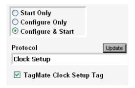
When the checkbox is checked, a tag will be marked as a clock setup tag. After starting the tag in this way, simply read it with a TagMate USB® and the clock will be updated.
