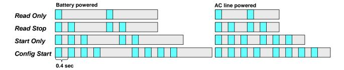
As the diagram shows, the repeat rate of the LED blink pattern is faster whenever the unit is connected to AC line power. The line-powered option is described later in the section. All tag processing operations that can be performed by the TagMate USB® from each of these modes are described in later sections.
