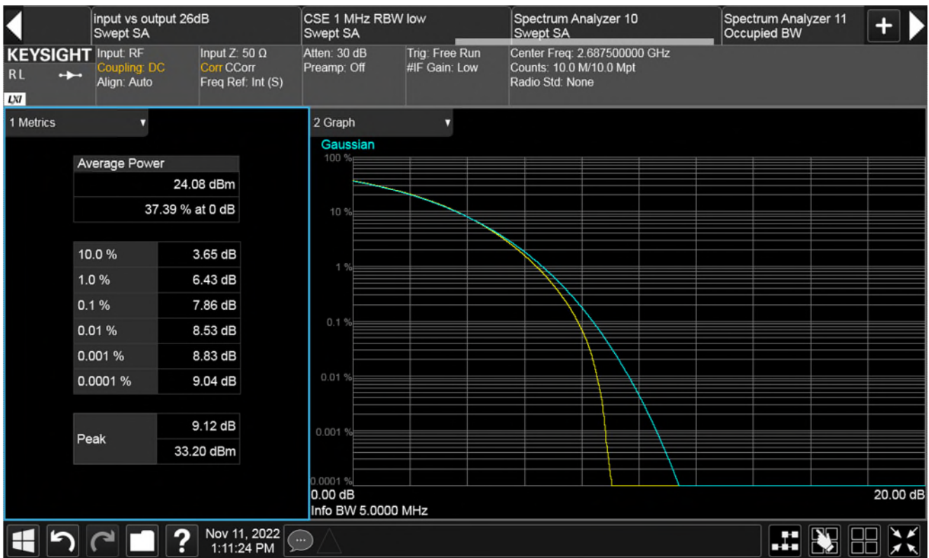
Plot of Peak to Average power ratio at determined f_0 in band 2496-2690 MHz
