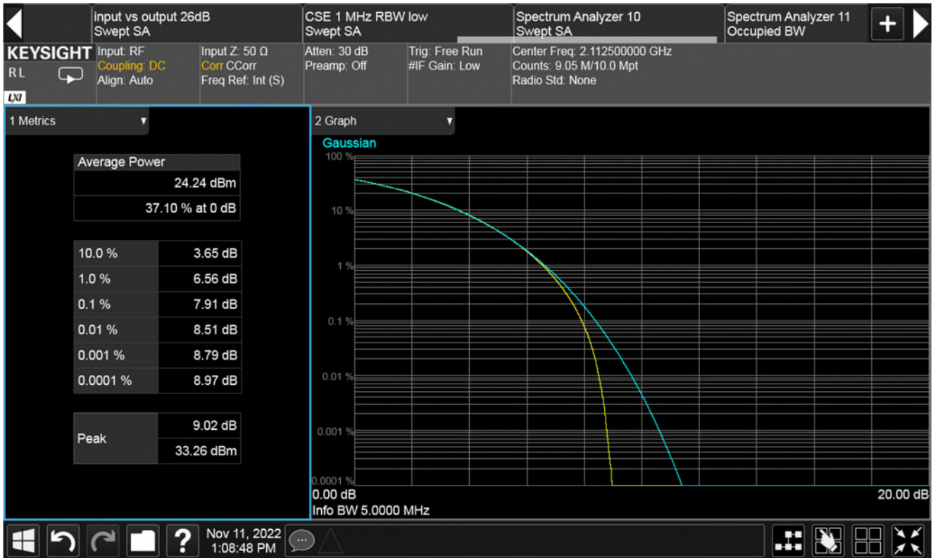
Plot of Peak to Average power ratio at determined f_0 in band 2110-2180 MHz
