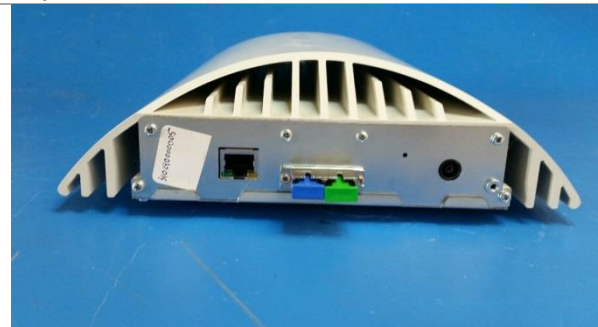
End #2: fiber optic and power
