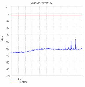
Start 30.0 MHz; Stop 800.0 MHz Ref 0 dBm; Ref Offset 13.0 dB; 10 dB/div RBW 100.0 KHz; VBW 100.0 KHz; Att 10 dB; Swp 200.0 mS Peak 729.417 MHz, -47.83 dBm Display Line; -13 dBm; ; Limit Test Passed Tested by jph 07/11/2006 09:05:01
