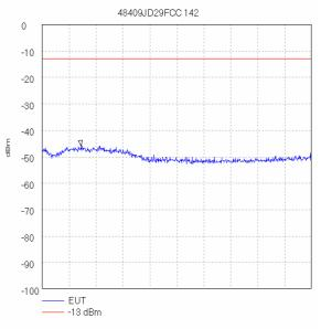
Start 25.0 GHz; Stop 30.0 GHz Ref 0 dBm; Ref Offset 13.0 dB; 10 dB/div RBW 1.0 MHz; VBW 1.0 MHz; Att 10 dB; Swp 100.0 mS Peak 25.717 GHz, -45.83 dBm Display Line: -13 dBm; ; Limit Test Passed Tested by jxh 07/11/2006 09:10:08
