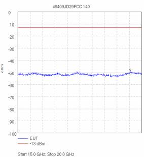
Start 15.0 GHz; Stop 20.0 GHz Ref 0 dBm; Ref Offset 13.0 dB; 10 dB/div RBW 1.0 MHz; VBW 1.0 MHz; Att 10 dB; Swp 100.0 mS Peak 19.533 GHz, -49.0 dBm Display Line: -13 dBm; ; Limit Test Passed Tested by jxh 07/11/2006 09:09:11
