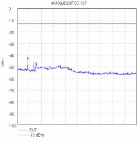
Start 1.0 GHz; Stop 5.0 GHz Ref 0 dBm; Ref Offset 13.0 dB; 10 dB/div RBW 1.0 MHz; VBW 1.0 MHz; Att 10 dB; Swp 80.0 mS Peak 1.34 GHz, -44.33 dBm Display Line: -13 dBm; ; Limit Test Passed Tested by jxh 07/11/2006 09:07:28
