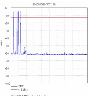
Start 800.0 MHz; Stop 1.0 GHz Ref 0 dBm; Ref Offset 13.0 dB; 10 dB/div RBW 100.0 kHz; VBW 100.0 kHz; Att 10 dB; Swp 50.0 mS Marker 834.667 MHz, -54.17 dBm Display Line: -13 dBm; ; Limit Test Passed Tested by jxh 07/11/2006 09:06:27
