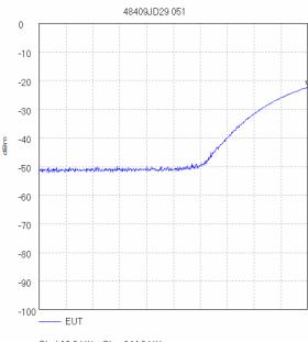
Start 10.0 MHz; Stop 244.8 MHz Ref 0 dBm; Ref Offset 10.0 dB; 10 dB/div RBW 2.0 MHz; VBW 3.0 MHz; Att 10 dB; Swp 50.0 mS Peak 244.8 MHz, -22.17 dBm Tested by jkh 14/09/2006 11:24:14
