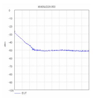
Start 3.0 GHz; Stop 5.0 GHz Ref 0 dBm; Ref Offset 11.0 dB; 10 dB/div RBW 2.0 MHz; VBW 3.0 MHz; Att 10 dB; Swp 50.0 mS Peak 3.0 GHz, -28.17 dBm Tested by jxh 14/09/2006 11:28:34
