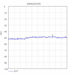
Start 5.0 GHz; Stop 10.0 GHz Ref 0 dBm; Ref Offset 11.0 dB; 10 dB/div RBW 2.0 MHz; VBW 3.0 MHz; Att 10 dB; Swp 100.0 mS Peak 8.742 GHz. -47.5 dBm Tested by jxh 14/09/2006 11:29:20
