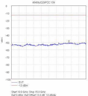
Start 10.0 GHz; Stop 15.0 GHz Ref 0 dBm; Ref Offset 13.0 dB; 10 dB/div RBW 1.0 MHz; VBW 1.0 MHz; Att 10 dB; Swp 100.0 mS Peak 13.85 GHz, -49.5 dBm Display Line: -13 dBm; ; Limit Test Passed Tested by jxh 07/11/2006 09:08:39
