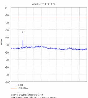
Ref 0 dBm; Ref Offset 13.0 dB; 10 dB/div RBW 1.0 MHz; VBW 1.0 MHz; Att 10 dB; Swp 80.0 mS Peak 1.627 GHz; -34.67 dBm Display Line: -13 dBm; ; Limit Test Passed Tested by jxh 07/11/2006 10:13:58
