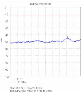
Ref 0 dBm; Ref Offset 13.0 dB; 10 dB/div RBW 1.0 MHz; VBW 1.0 MHz; Att 10 dB; Swp 100.0 mS Peak 24.05 GHz, -44.33 dBm Display Line: -13 dBm; ; Limit Test Passed Tested by jxh 07/11/2006 10:15.49
