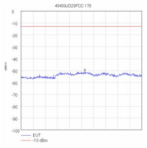
Start 5.0 GHz; Stop 10.0 GHz Ref 0 dBm; Ref Offset 13.0 dB; 10 dB/div RBW 1.0 MHz; VBW 1.0 MHz; Att 10 dB; Swp 100.0 mS Peak 7.642 GHz, -50.83 dBm Display Line; -13 dBm; ; Limit Test Passed Tested by jxh 07/11/2006 10:14:23
