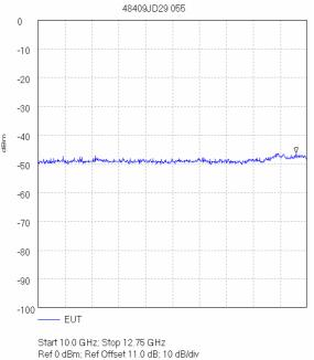
Ref 0 dBm; Ref 0ffset 11.0 dB; 10 dB/div RBW 2.0 MHz; VBW 3.0 MHz; Att 10 dB; Swp 55.0 mS Peak 12.635 GHz, -46.17 dBm Tested by jxh 14/09/2006 11:30:06
