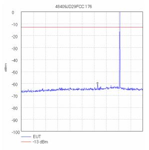
Start 30.0 MHz; Stop 1.0 GHz Ref 0 dBm; Ref Offset 13.0 dB; 10 dB/div RBW 100.0 kHz; VBW 100.0 kHz; Att 10 dB; Swp 250.0 mS Marker 637.867 MHz, -61.0 dBm Display Line: -13 dBm; ; Limit Test Passed Tested by jxh 07/11/2006 10:13:14
