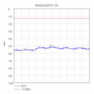
Start 5.0 GHz; Stop 10.0 GHz Ref 0 dBm; Ref Offset 13.0 dB; 10 dB/div RBW 1.0 MHz; VBW 1.0 MHz; Att 10 dB; Swp 100.0 mS Peak 7.425 GHz, -50.33 dBm Display Line: -13 dBm; ; Limit Test Passed Tested by jxh 07/11/2006 09:08:07
