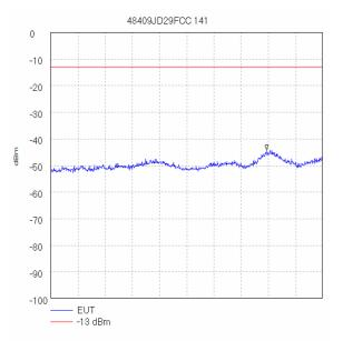
Start 20.0 GHz; Stop 25.0 GHz Ref 0 dBm; Ref Offset 13.0 dB; 10 dB/div RBW 1.0 MHz; VBW 1.0 MHz; Att 10 dB; Swp 100.0 mS Peak 23.967 GHz, -44.17 dBm Display Line: -13 dBm; ; Limit Test Passed Tested by jxh 07/11/2006 09:09.39
