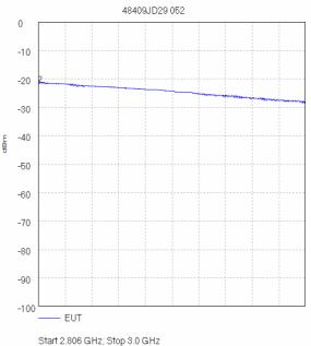
Start 2.806 GHz; Stop 3.0 GHz Ref 0 dBm; Ref Offset 11.0 dB; 10 dB/div RBW 2.0 MHz; VBW 3.0 MHz; Att 10 dB; Swp 50.0 mS Peak 2.806 GHz, -21.17 dBm Tested by jxh 14/09/2006 11:26:14
