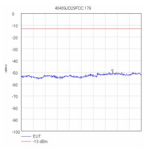
Start 10.0 GHz; Stop 15.0 GHz Ref 0 dBm; Ref Offset 13.0 dB; 10 dB/div RBW 1.0 MHz; VBW 1.0 MHz; Att 10 dB; Swp 100.0 mS Peak 13.8 GHz, -49.67 dBm Display Line; -13 dBm;; Limit Test Passed Tested by jxh 07/11/2006 10:14:48
