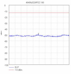
Start 15.0 GHz; Stop 20.0 GHz Ref 0 dBm; Ref Offset 13.0 dB; 10 dB/div RBW 1.0 MHz; VBW 1.0 MHz; Att 10 dB; Swp 100.0 mS Peak 17.442 GHz, -49.0 dBm Display Line: -13 dBm; ; Limit Test Passed Tested by jxh 07/11/2006 10:15:14
