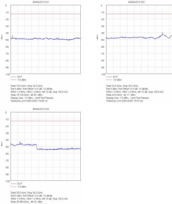
Display Line: -13 dBm; ; Limit Test Passed Tested by JXH 03/01/2007 15:57:25
