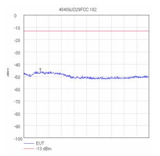
Start 25.0 GHz; Stop 30.0 GHz Ref 0 dBm; Ref Offset 13.0 dB; 10 dB/div RBW 1.0 MHz; VBW 1.0 MHz; Att 10 dB; Swp 100.0 mS Peak 25.658 GHz, -45.33 dBm Display Line: -13 dBm; ; Limit Test Passed Tested by jxh 07/11/2006 10:16:12
