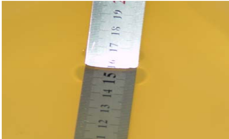
Liquid depth for SAR Measurement
