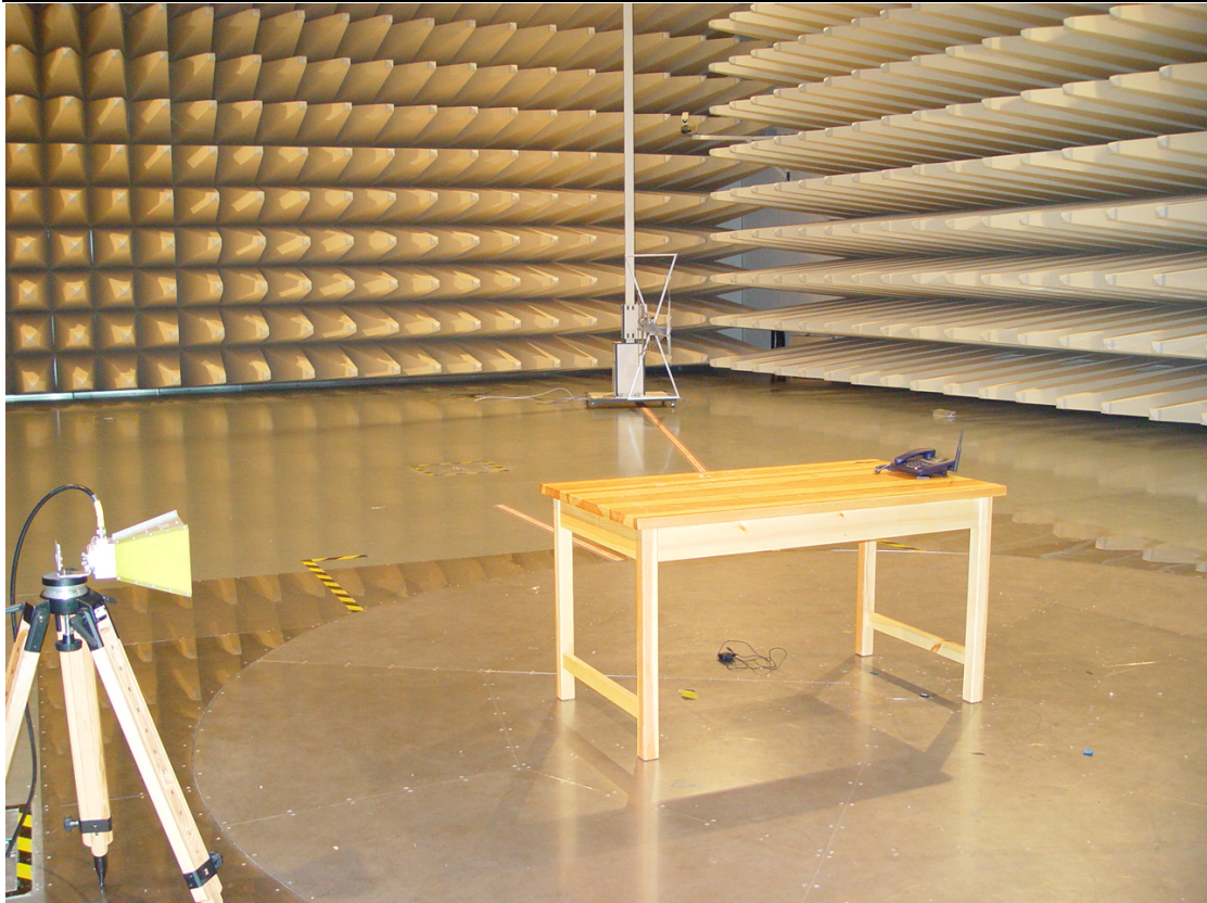
Pic 3 Radiated Emissions Test Setup
