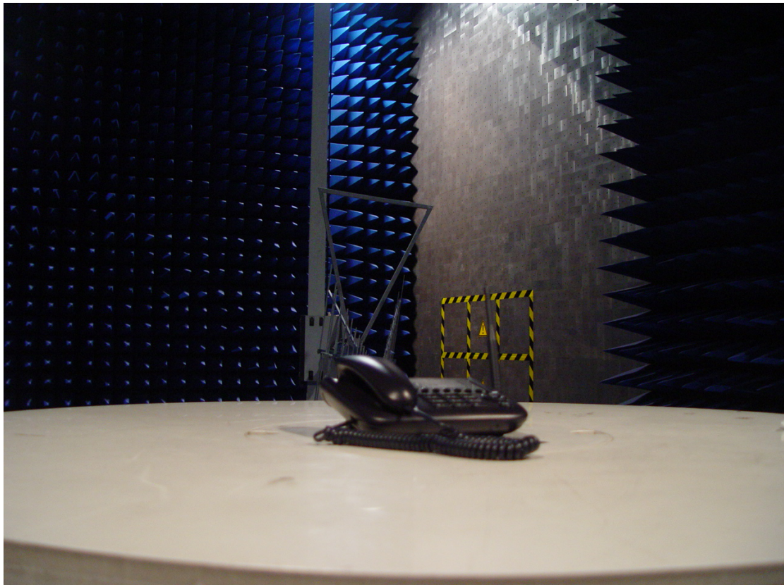
Pic 2 Radiated Spurious Emissions Test Setup
