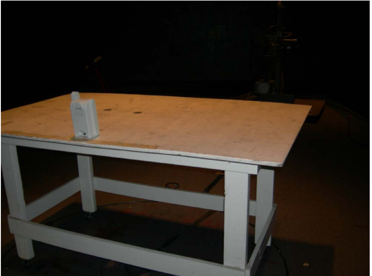
Figure 2: Test Set Up – Radiated Emissions View 2
