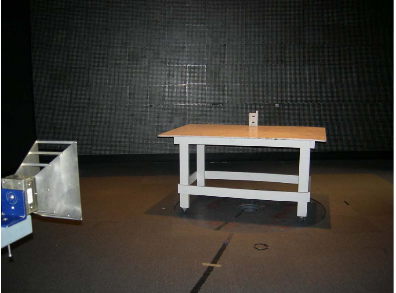
Figure 1: Test Set Up – Radiated Emissions
