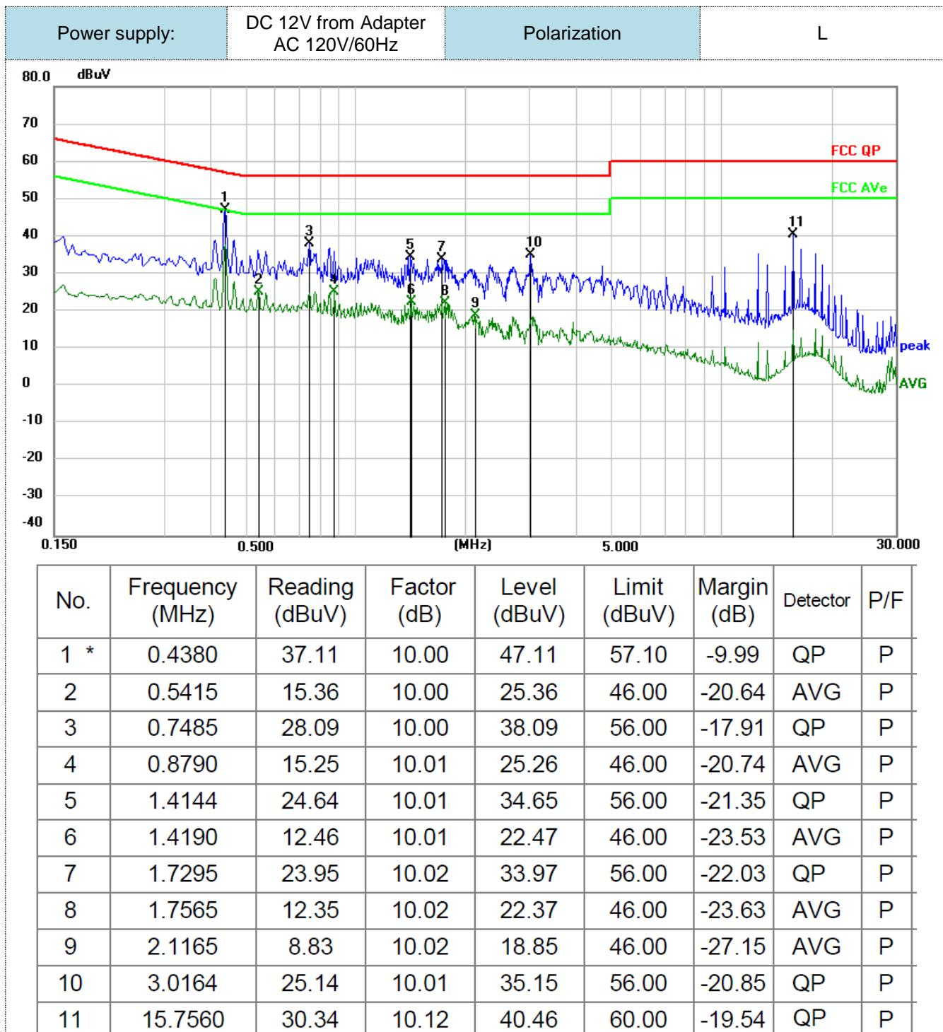
Note: Note:1).QP Value (dB $\mu$ V)= QP Reading (dB $\mu$ V)+ Factor (dB)
