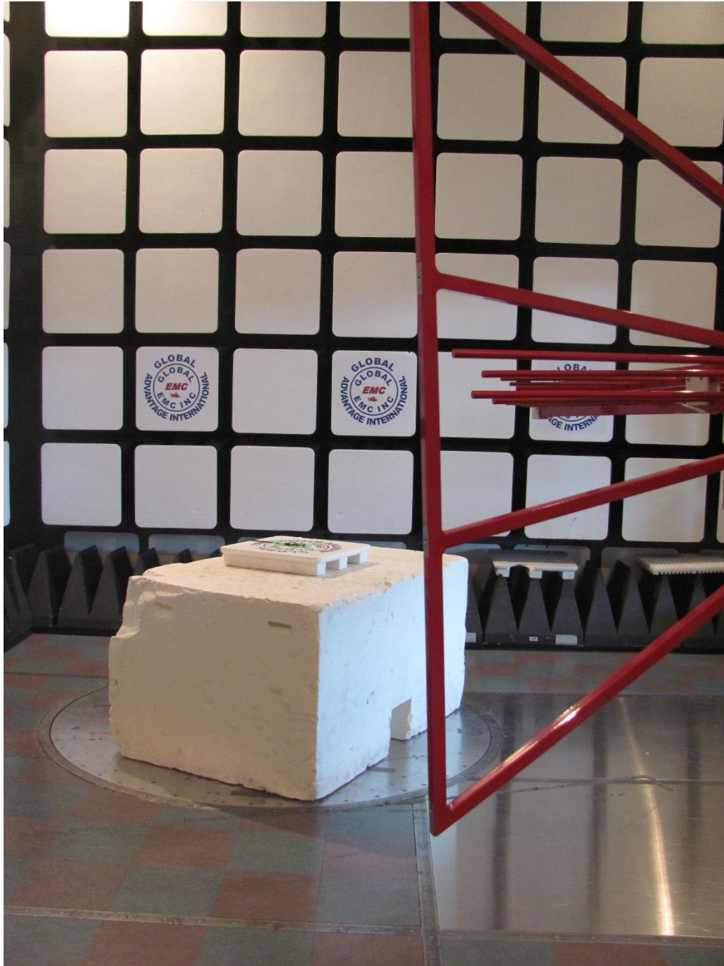
Figure 2 – Radiated Emissions Setup – Photo 2
