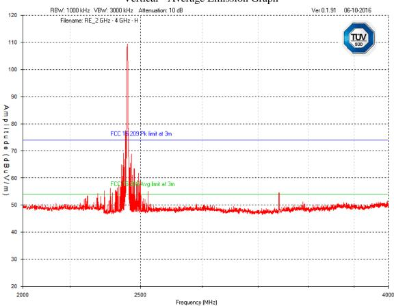
Note: See Final Measurements and Results section starting on page 52 for measurements. Emissions at 3.2 GHz is a modulation artifact of the EUT; its Average emission levels is derived from Peak emission; see emission table on page 52 for details.
