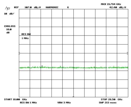
Plot was taken at 1 meter distances. All emissions shown were instrument noise floor of measurement instrument. No emissions were found in this frequency range.
