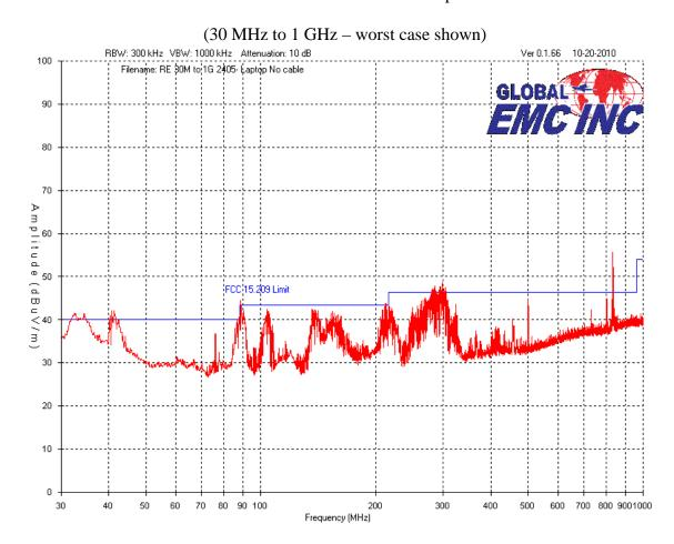
Note: Receive mode was identical, with the exception of the frequency shown between 800 MHz and 828 MHz not being present.
