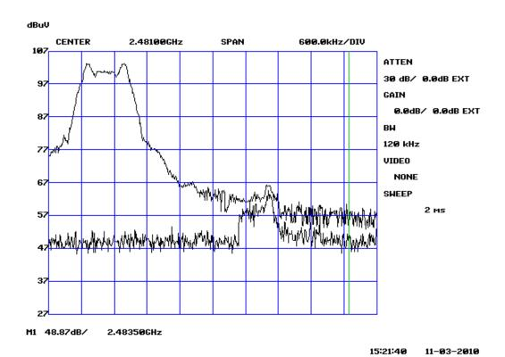
Fundamental centered at 2479 MHz, marker (green line) at 2483.5 MHz.
