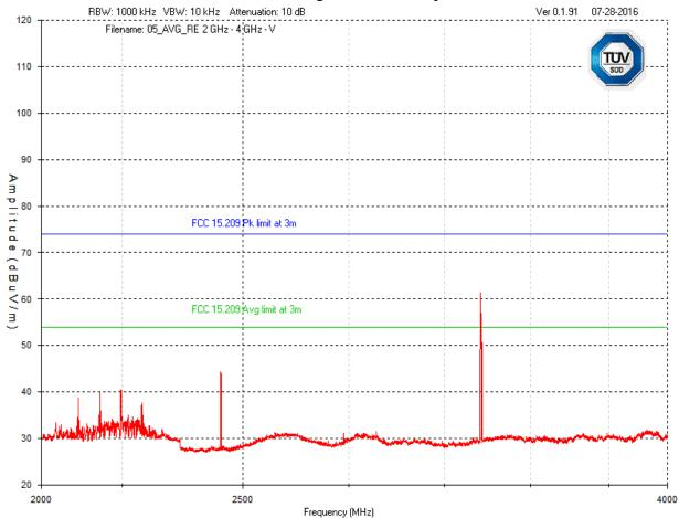
Note: See Final Measurements and Results section starting on page 53 for measurements. Emissions at 3.2 GHz is a modulation artifact of the EUT; its Average emission levels is derived from Peak emission; see emission table on page 53 for details.
