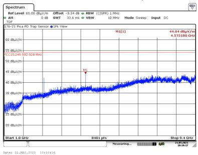
A.4.2. Measurement Results - Vertical Antenna, X Axis
