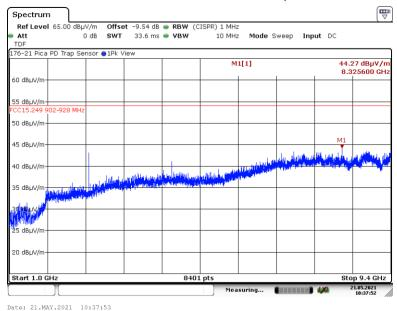
A.4.6. Measurement Results – Vertical Antenna, Z Axis
