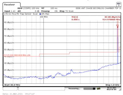
A.3.2. Measurement Results - Vertical Antenna, X Axis
