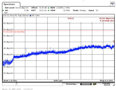
A.4.4. Measurement Results - Vertical Antenna, Y Axis
