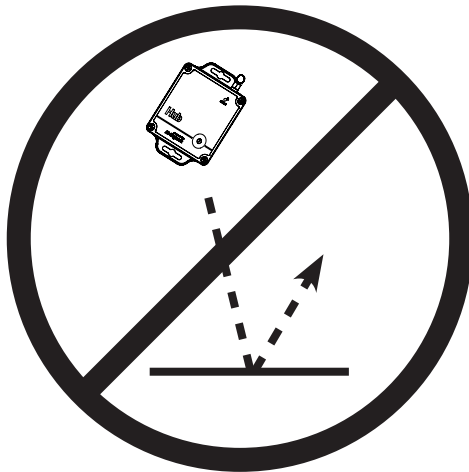
Prevent Unit Fall Damage
