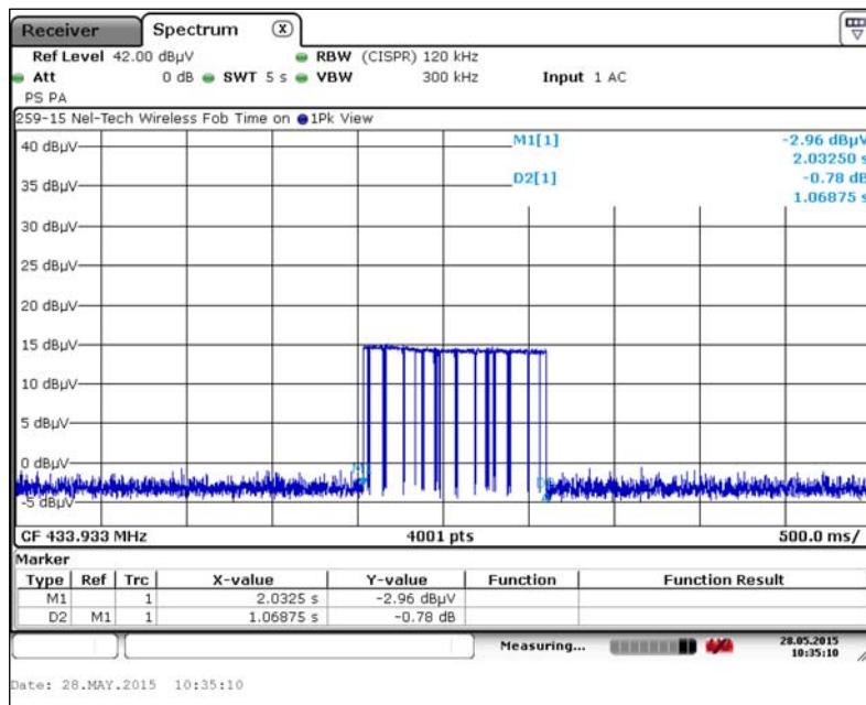
6.2.2. Requirement: A transmitter activated automatically shall cease transmission within 5 seconds after activation (Section 15.231(a)(2)).
