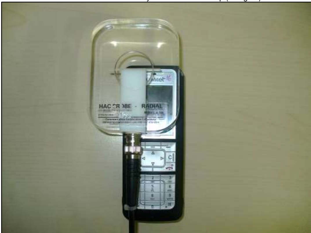
Photo 4: Radial field intensity measurement set-up (0 degree)
