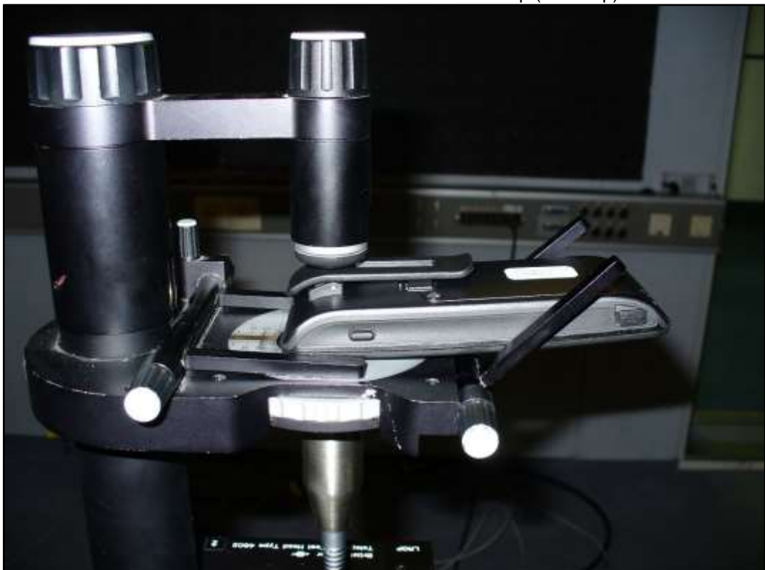
Photo 2: Volume control measurement set-up (close-up)
