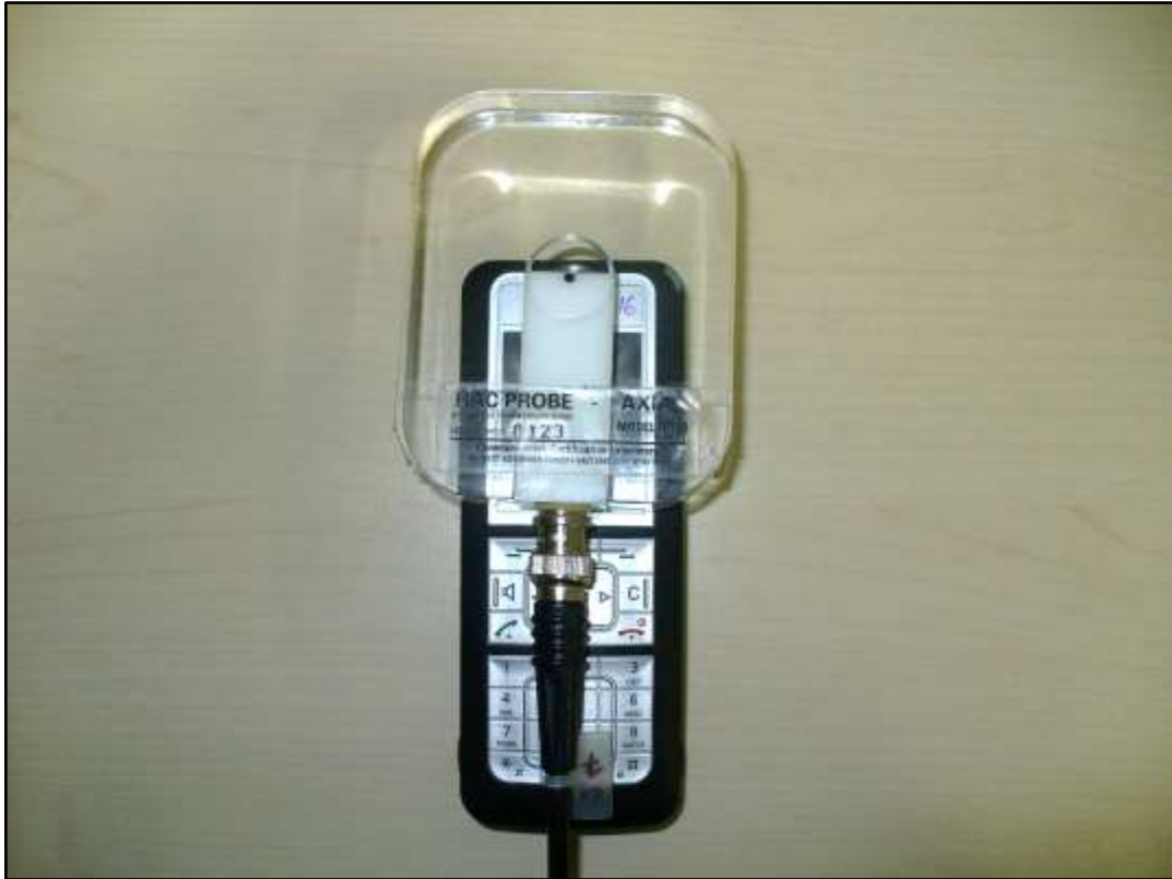
Photo 4: Radial field intensity measurement set-up (0 degree)
