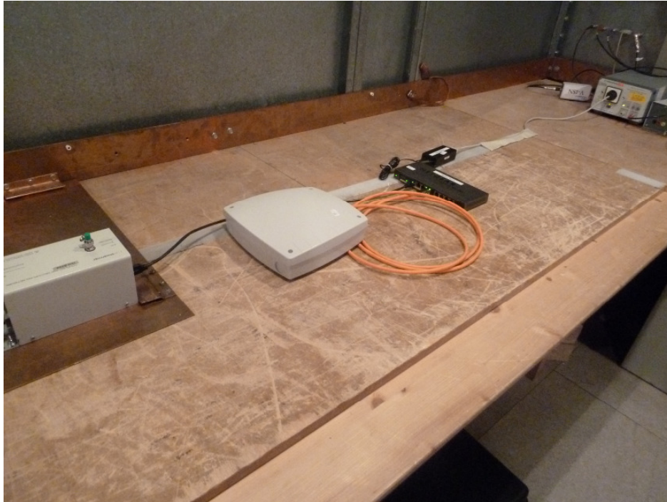
Photo 1: Power Line Conducted Emission Test
