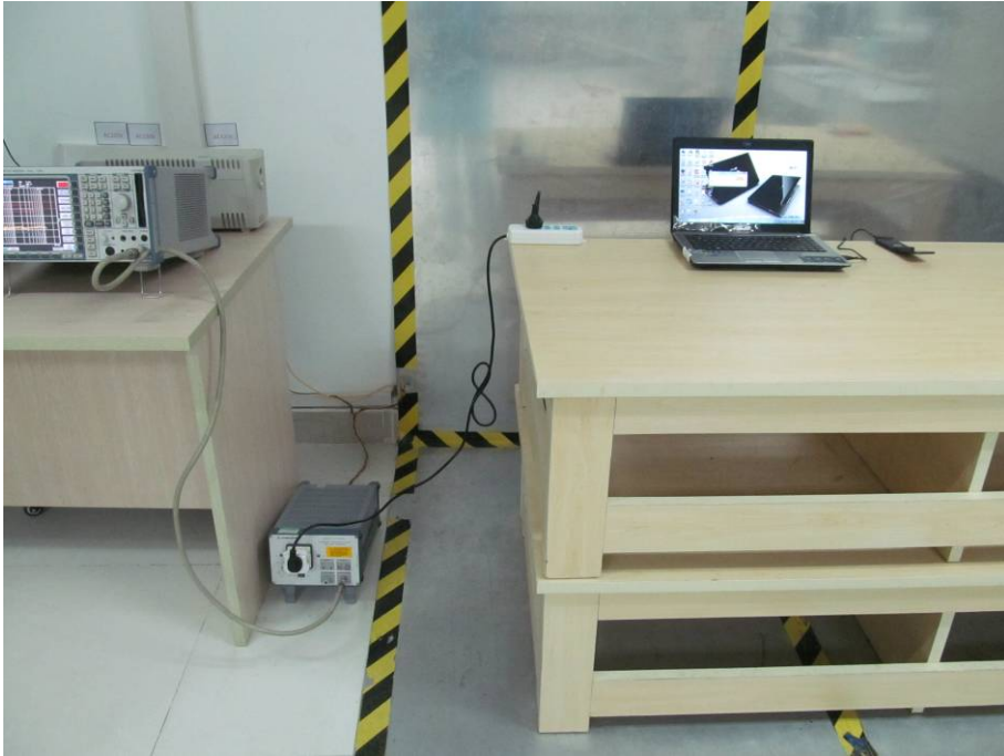
FCC RADIATED EMISSION TEST SETUP
