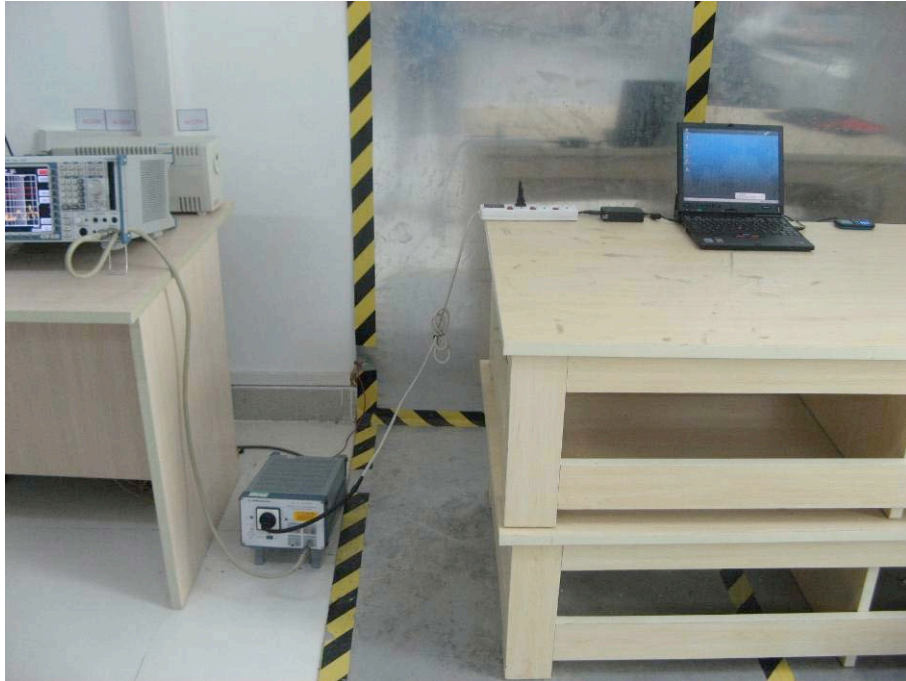
FCC LINE CONDUCTED EMISSION TEST SETUP
