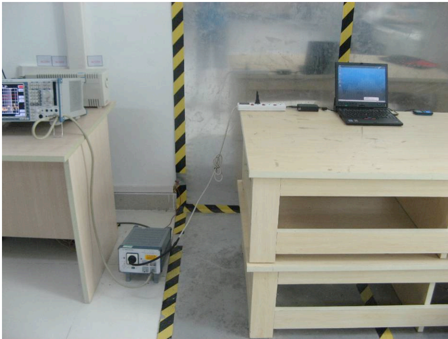
FCC LINE CONDUCTED EMISSION TEST SETUP
