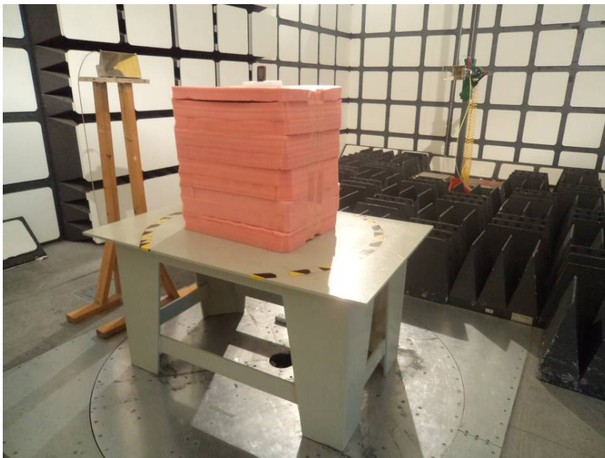
Radiated Emissions Test View (Above 1 GHz)
