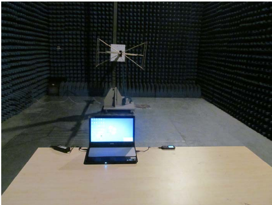
FCC RADIATED EMISSION TEST SETUP
