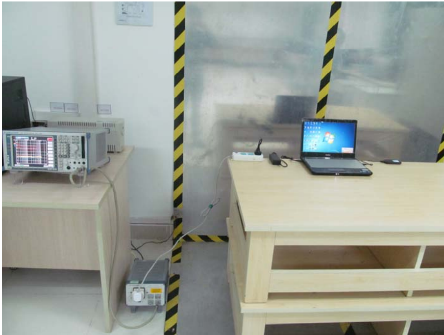
FCC LINE CONDUCTED EMISSION TEST SETUP
