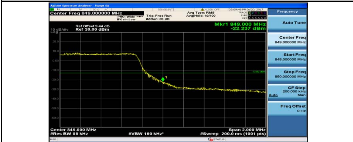
(Channel Bandwidth: 5 MHz)_HCH_16QAM_25RB#0
