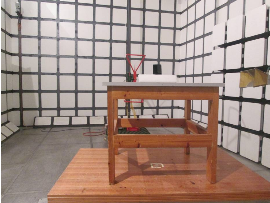
Radiated Emissions Test View (Below 1 GHz)
