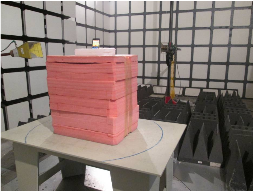
Radiated Emissions Test View (Above 1 GHz)
