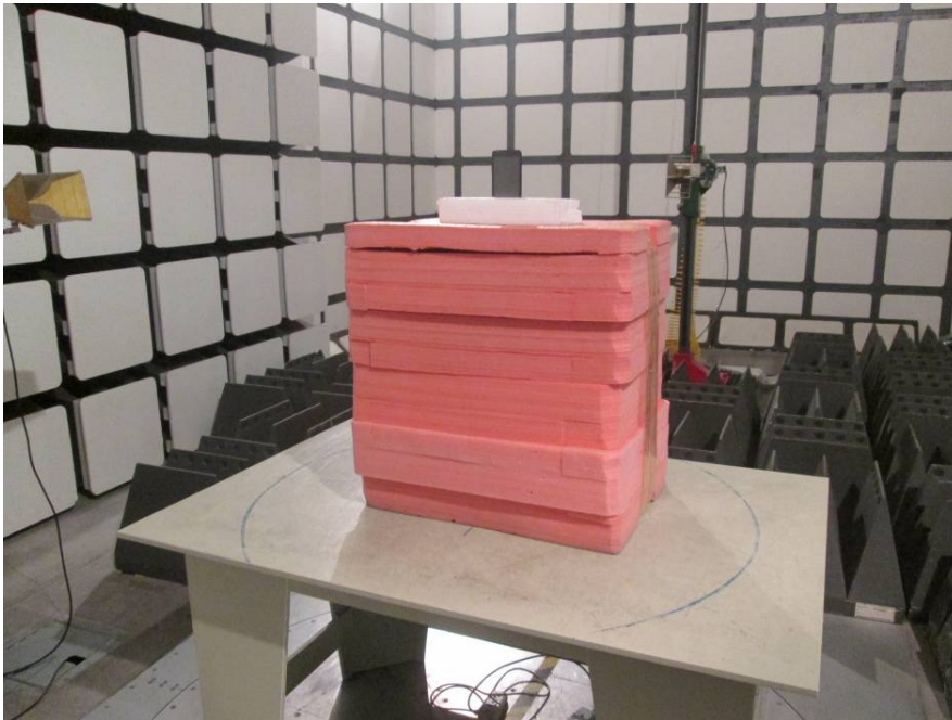
Radiated Emissions Test View (Above 1 GHz)
