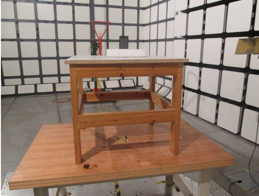
Radiated Emissions Test View (Below 1 GHz)
