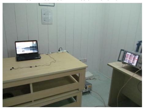
FCC RADIATED EMISSION TEST SETUP
