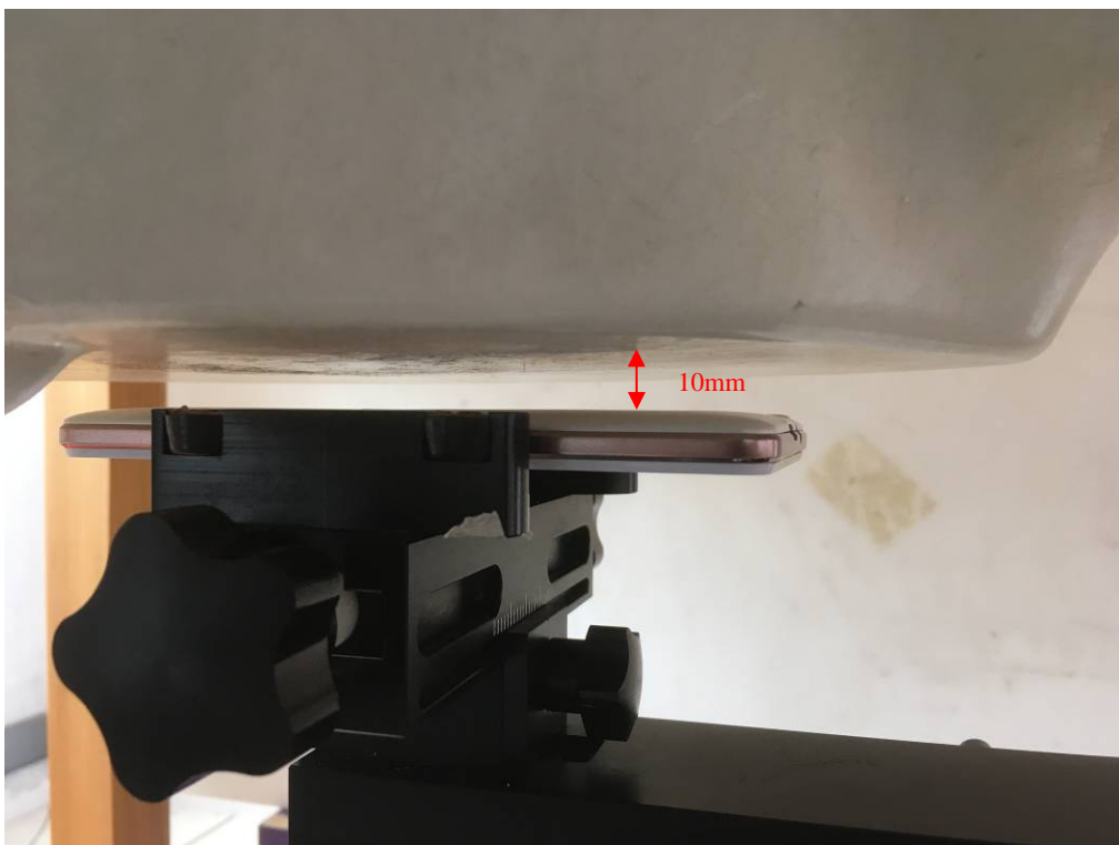
Body Worn & Body Back Setup Photo (10mm)
