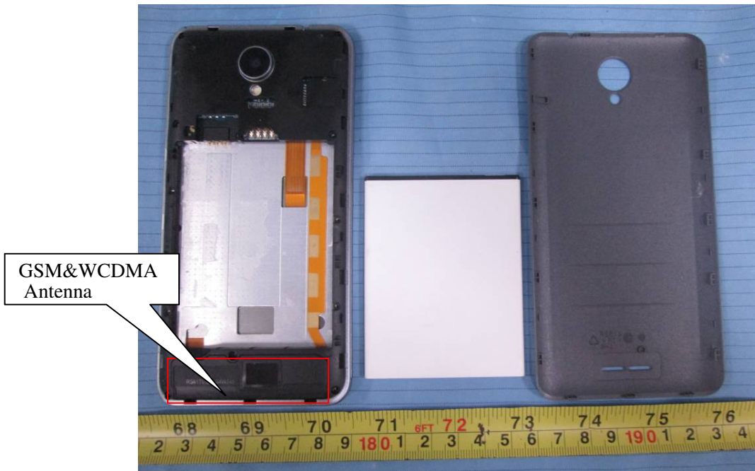
EUT – Cover off View 1
