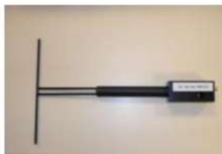
Figure 1 – Satimo COMOSAR Validation Dipole
