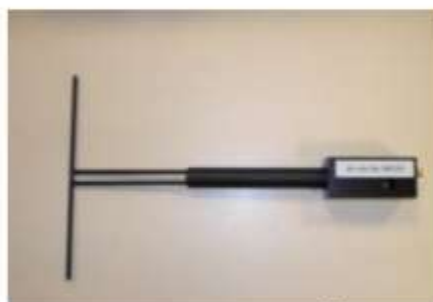
Figure 1 – Satimo COMOSAR Validation Dipole
