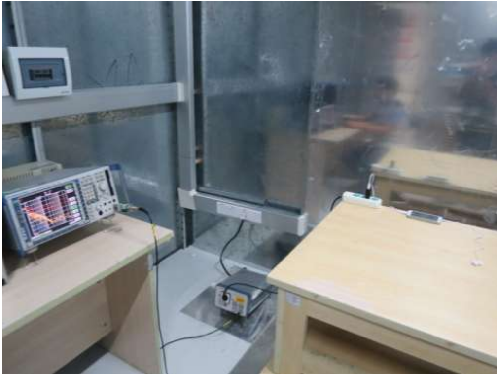
FCC RADIATED EMISSION TEST SETUP
