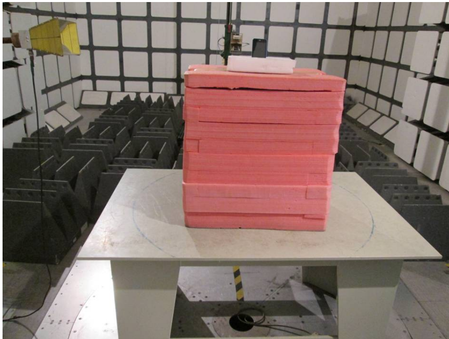
Radiated Emissions Test View (Above 1 GHz)
