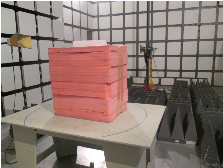
Radiated Emissions Test View (Above 1 GHz)
