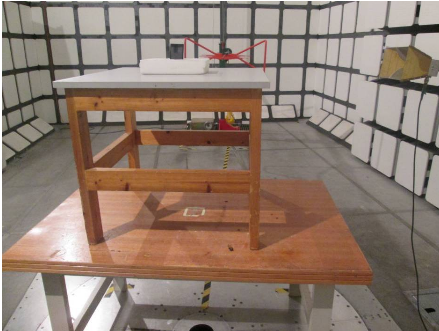
Radiated Emissions Test View (Below 1 GHz)
