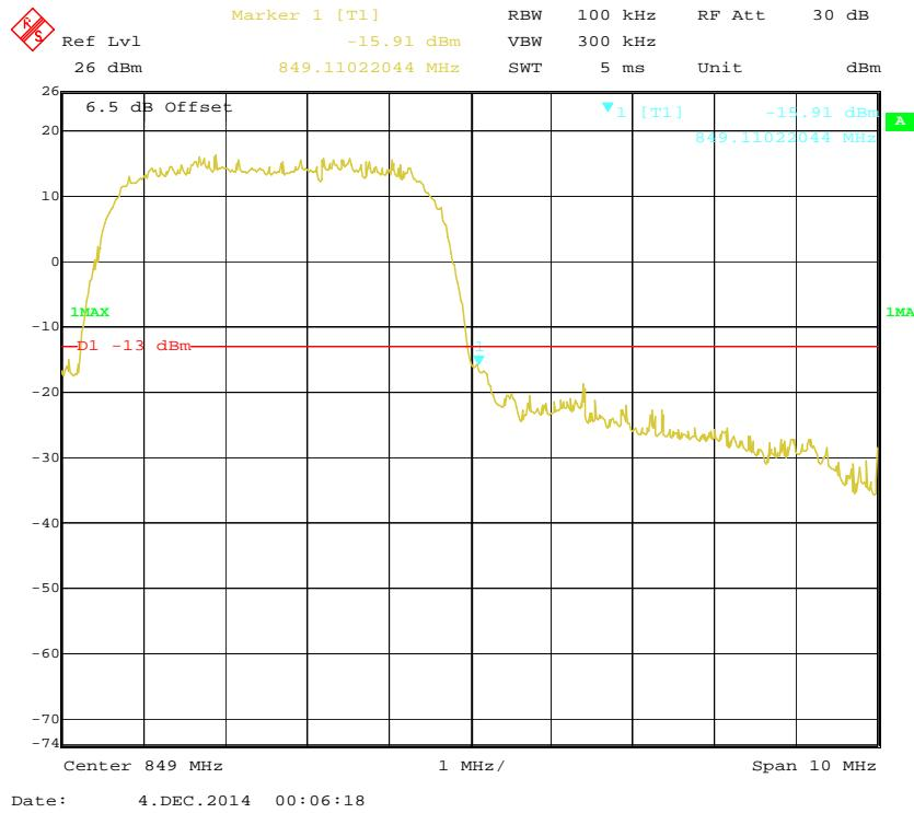
**PCS Band, Left Band Edge for GSM (GMSK) Mode**
