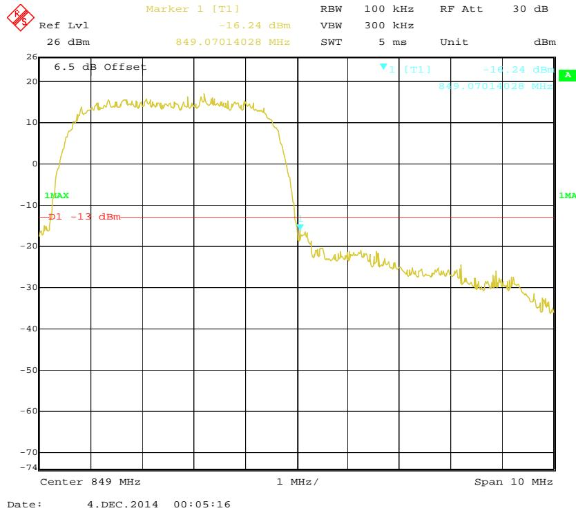
**Cellular Band, Left Band Edge for HSUPA (BPSK) Mode**
