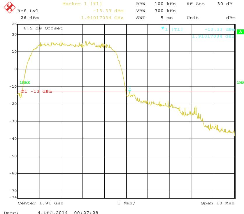
**PCS Band, Left Band Edge for HSUPA (BPSK) Mode**
