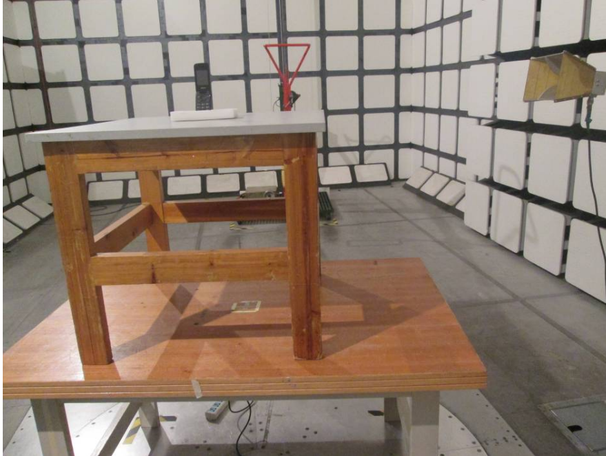
Radiated Emissions Test View (Below 1 GHz)
