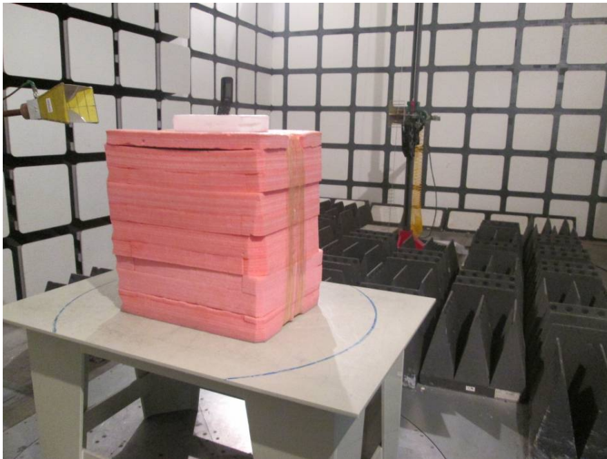
Radiated Emissions Test View (Above 1 GHz)
