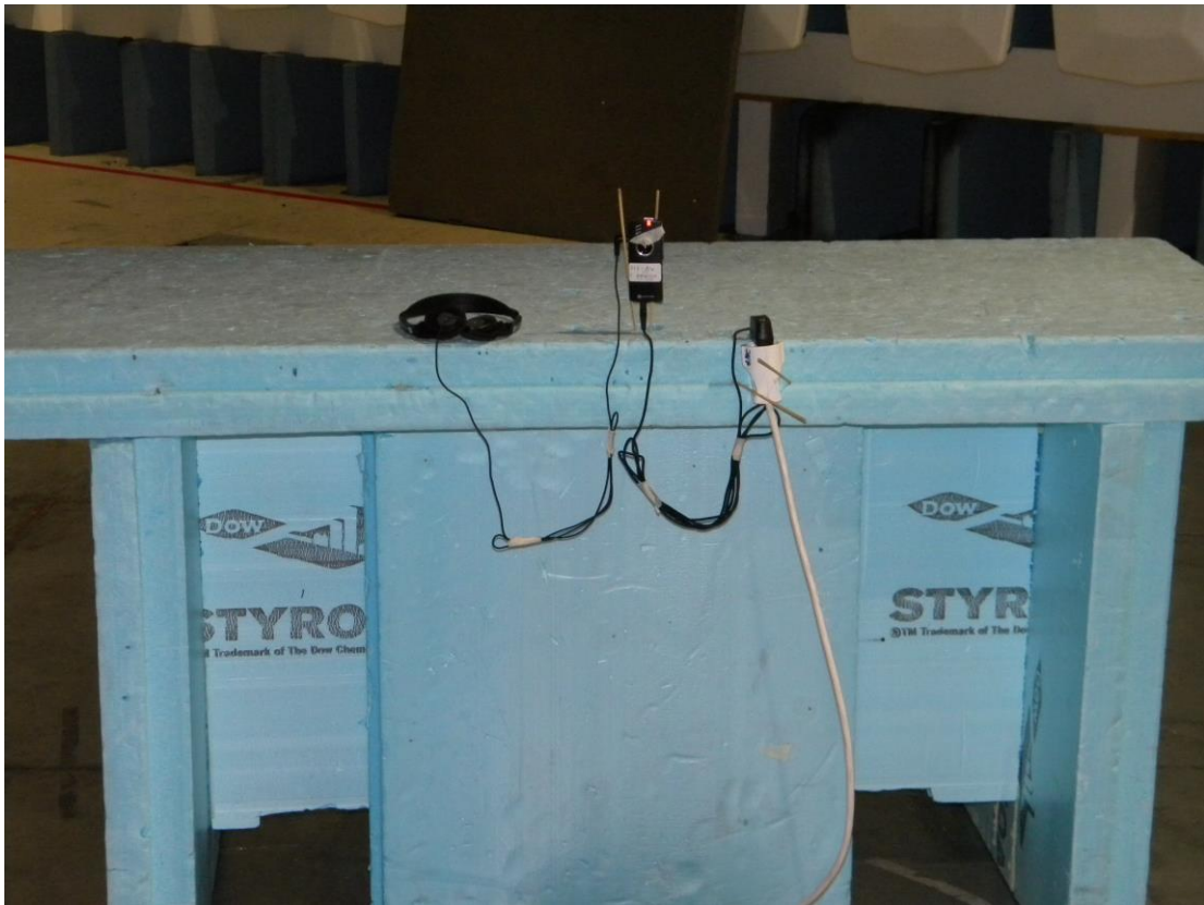
Photograph 1. Spurious radiated emissions test setup
