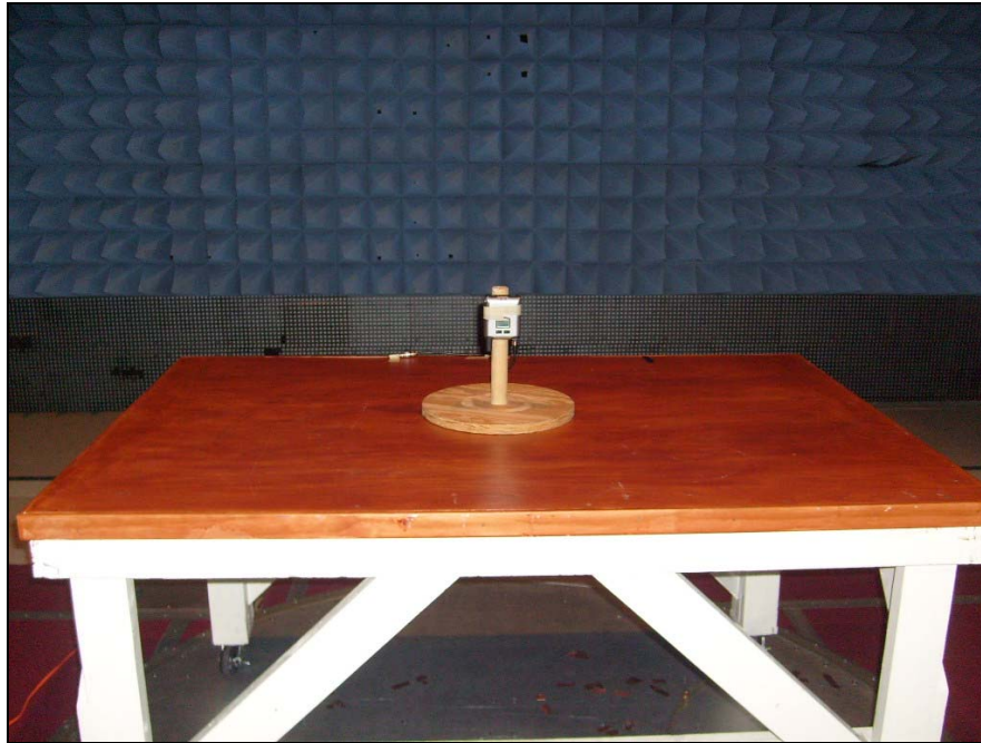
Photograph 2. Various Radiated Measurements, Test Setup
