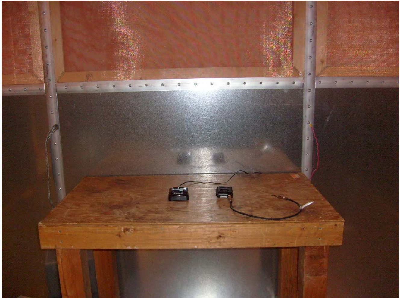
Photograph 2. Conducted Emissions Test Setup
