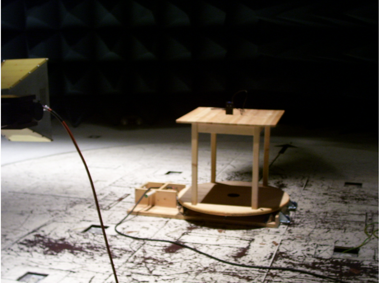
Photograph 2. Test Equipment and setup for various Radiated Measurements
