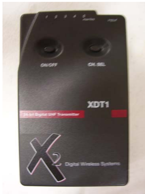
Photograph 1. X2 Digital Wireless 900 MHz ISM Band Digital Audio Transmitter
