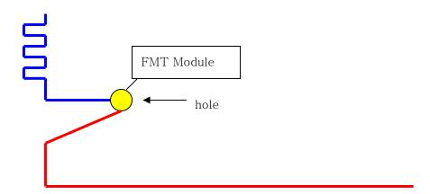
The above yellow via hole is under the SD slot. So you cannot find the picture. Please refer to the attached PCB film file.
