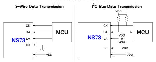
The NS73 has two types of serial data interface: 3-wire and I<sup>2</sup>C bus.
