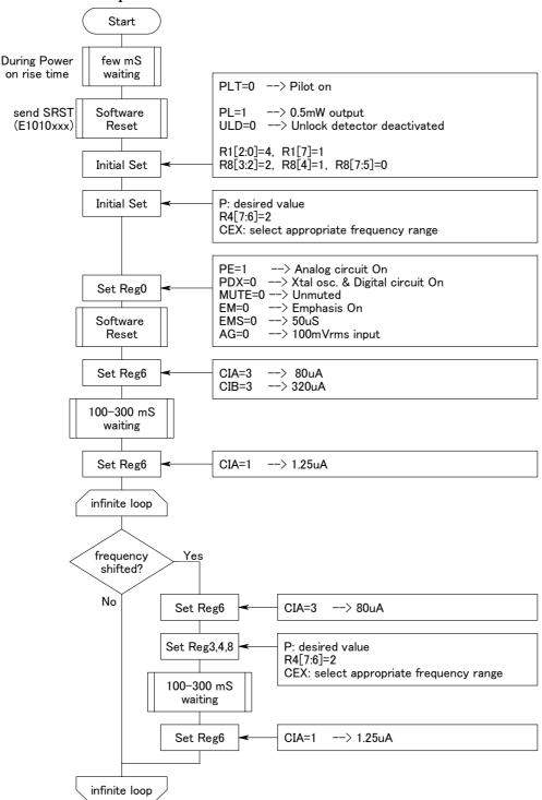
NS73 has power on reset circuit. Because this function works, has to wait for a few milli-seconds until VDD reaching specified value.
