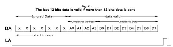
The last 12 bits (12 bits before latch pulse) are acceptable as valid data.
