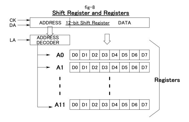
Although the software-reset function is assigned to the address 14, no register for this function exists.
