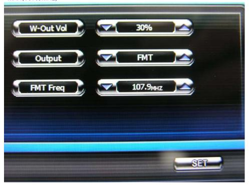
\* The tuning range is 88.1 ~ 107.9MHz, (100KHz step) setting as program firmware the frequency can be controlled manually. the frequency range is 88.1~107.9
