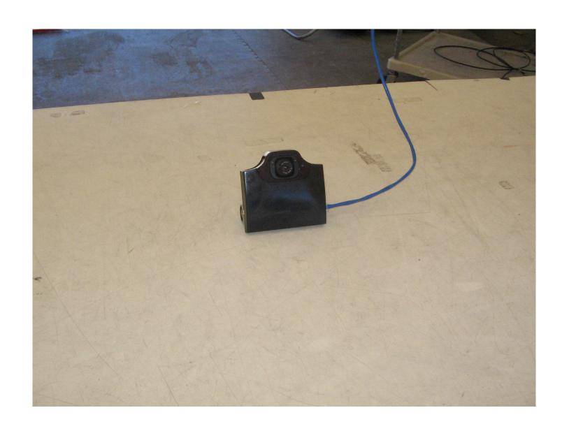
Radiated Emissions Measurement (Front View) Setup
