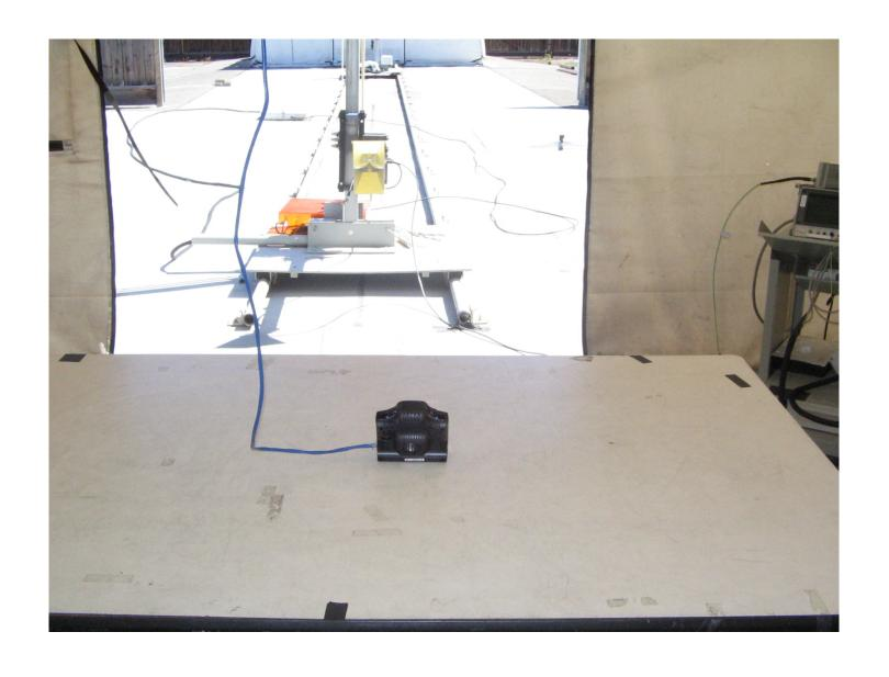
Radiated Emissions Measurement (Rear View) Setup
