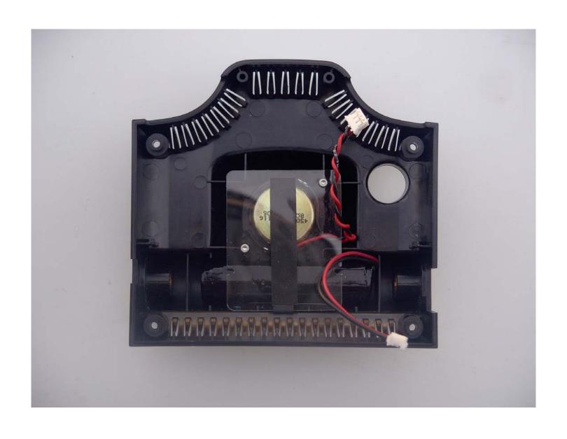
Bottom Cover View "Disconnected from Main PCB"
