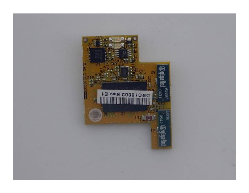
WLAN PCB Top View
