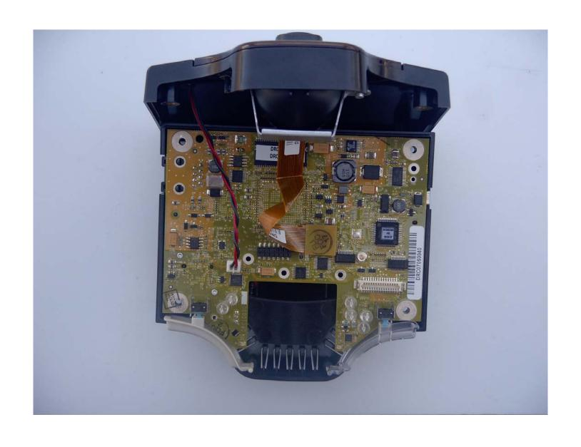
Main PCB Top View "Connected to Top Cover"
