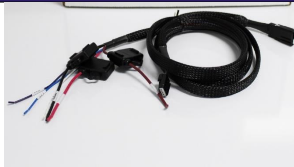
Vehicle Interface Cable with inline fuses: Red and Black wires = 5-amp fuses Brown wire = 1-amp fuse
